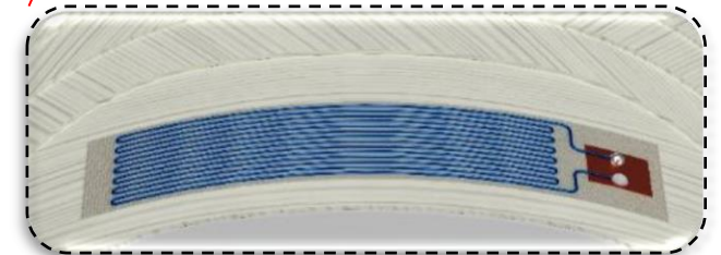
Pressure vessel with integrated strain gauges
